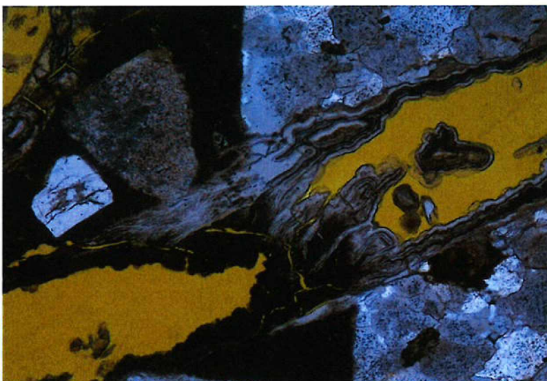
ASR gel in scheur korrel 100X PPL
