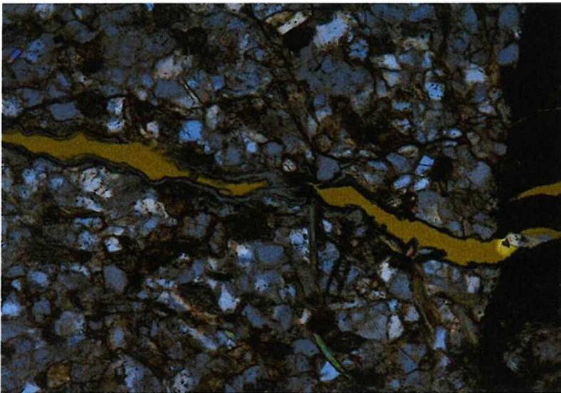
ASR gel in scheur korrel (100X PPL)
